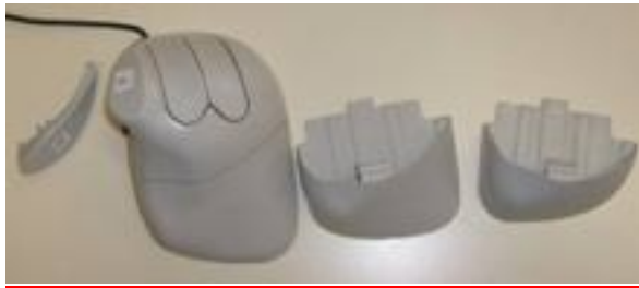
Figura 1 – Mouse ortopédico – Orthomouse
