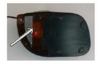
Other features to be appreciated: the special "antiskidding" texture, the scroll buttons with direct auctioning, the use of switches with lower mechanical resistance, the location of the optical sensor to allow precision with minimal "surface travel".
